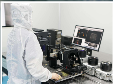
Cylindrical lens detection of 6-inch laser interferometer
